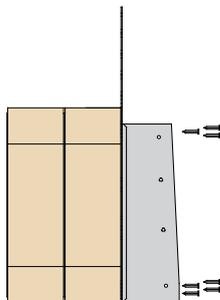
Face nail to top and bottom chords using 14No 3.4 x 35mm square twist nails in total.
