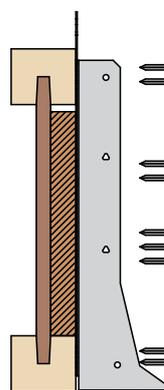
Fill all round and triangular nail holes to header and backer face with 3.4 x 35mm square twist nails.
