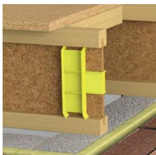
Place the Hi-Vis Gripper onto one end of the I-Joist to be built into the masonry. Push fit until it is fully engaged. Ensure it tightly abuts the I-Joist web and that both ends of the Hi-Vis Gripper tightly abut the I-Joist flanges.
