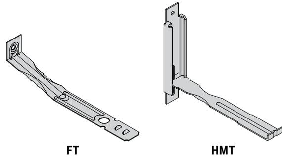
Cullen standard wall ties FT-50, 75 & 100 accommodate maximum differential movement of 25mm and therefore can be used up to eaves level on a 2 storey for solid timber joists and up to 3 storey for EWP joist floors. For 3 storey solid timber joists and 4 storey EWP joists you will now require the Cullen High Movement Tie (HMT).
