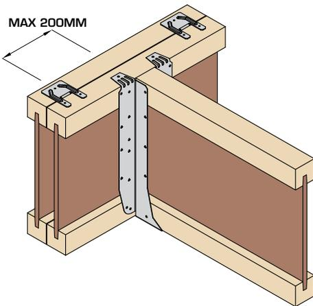
Installation either side of incoming point load to be maximum 200mm from joist edge.
