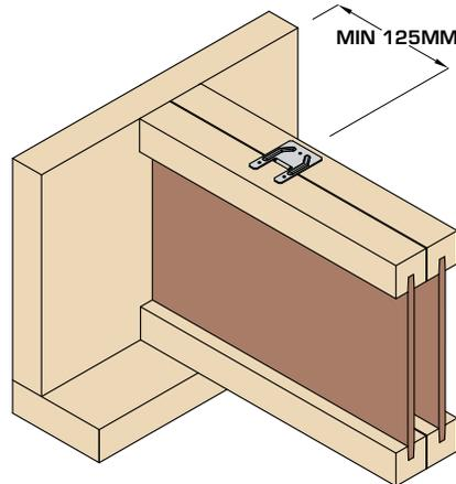
Installation on joist end to be minimum 125mm away from the end of the joist to allow adequate space for fixing.
