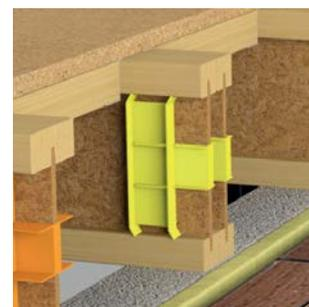
Second Hi-Vis Gripper abuts first to provide an air tight seal.
