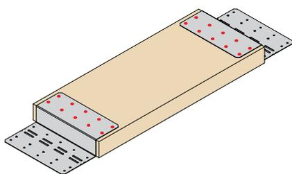
Nail support bracket to timber bracing shelf (min C16 grade) with 10No fixings per bracket (3.4 x 35mm square twist nails).
