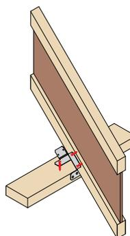
Position the I-Joist rafter and fix into the bottom flange with 2No 3.4 x 35mm square twist nails. On the same side fix into the top of the wall plate with 2No 3.4 x 35mm square twist nails.
