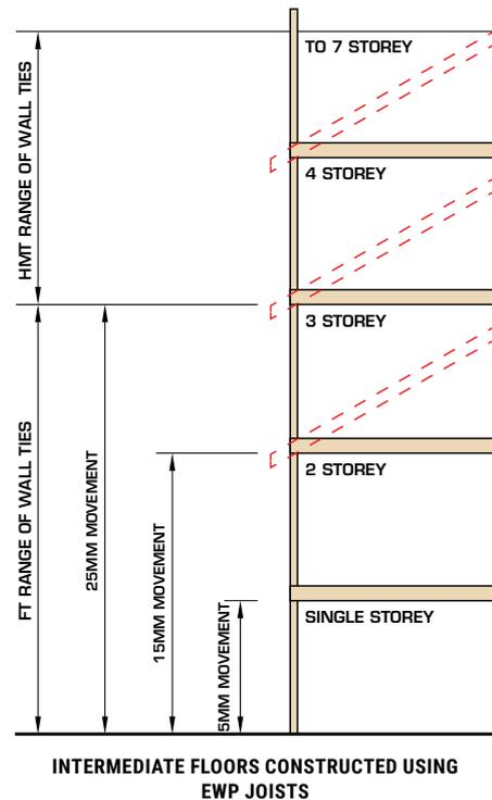
The above information is for guidance only, it states the maximum allowed movement of the Cullen timber frame wall tie range. For specific tie fixings please refer to the Building Engineer and/or section 6.2 of NHBC standards.
