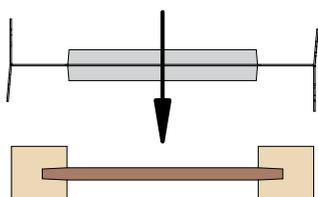
Lay I-Joist flat and mark location of I-Clips, press clips into position on top face of I-Joist.
