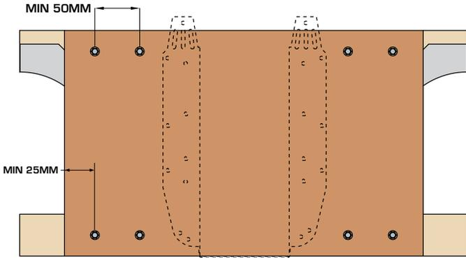
18mm plywood should be fixed to the face of the open web joist with 4No PSTS 6.5mm into the top chord and 4No PSTS 6.5mm into the bottom chord.
