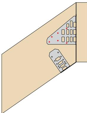
Wipe round the top side flange at the appropriate crease line and fill all the nail holes into the incoming joist. Minimum 4No 3.4 x 35mm square twist nails.
