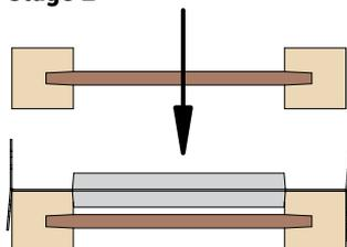
Position second ply of multiple joist on top of I-Clips and tap together with a hammer to ensure a tight fit.
