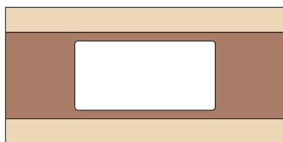
Using the SHI plate as a template, drill 4No holes and cut inner aperture to suit.
