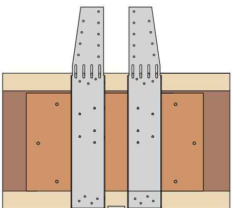
Position hanger flush with underside of joist.
