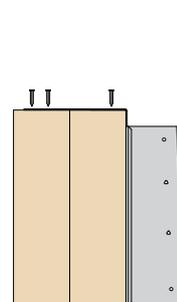
Nail top tabs into top chord of joist – Min 2No 3.4 x 35mm square twist nails into rear ply and 1No 3.4 x 35mm square twist nail into front ply per leg.
