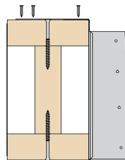
Nail top tabs into top chord of joist – Min 2No 3.4 x 35mm square twist nails into rear ply and 1No 3.4 x 35mm square twist nail into front ply per leg.
