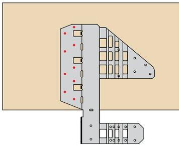
Face fix VRC to solid header using 9No 3.4 x 35mm square twist nails. Adjust angle of base plate if slope is required.
