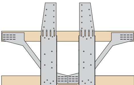
Position hanger flush with underside of joist.
