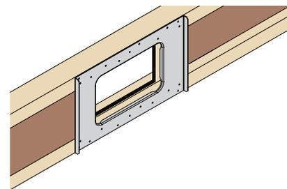
Fix the SHI plates to the I-Joist with 22No 3.4 x 35mm square twist nails per plate.
