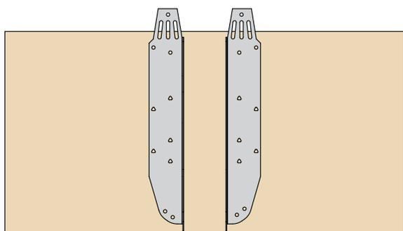
Position hanger against face of joist with locating tab tight to underside of joist.
