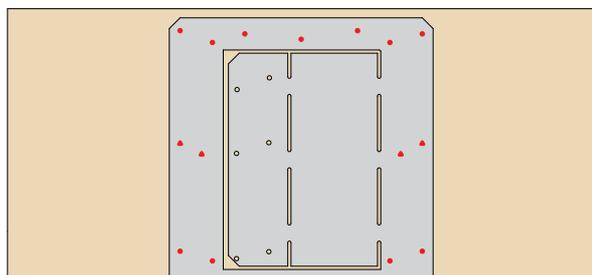
Please ensure that 1No inner nail hole (indicated in red) and 1No outer nail hole (indicated in red) are filled on the underside with 3.4 x 35mm square twist nails.
