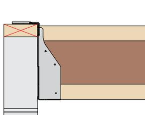
Do not install the hanger onto a timber wall plate.
