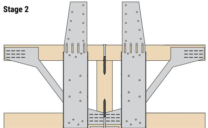
Position hanger against face of Open Web Joist with locating tab tight to underside of joist.
