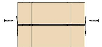
Fix OW-Clips to top and bottom chords of the multiple joist using 2No 3.4 x 35mm square twist nails per clip, ensuring that joists are fitted tightly together.
