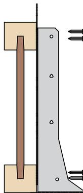
Face nail to top and bottom flanges using 8No 3.4 x 35mm square twist nails in total.
