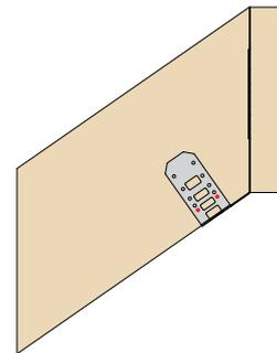
Wipe up the bottom side flange at the appropriate crease line and fill the 2No nail holes closest to the bend line with 3.4 x 35mm square twist nails.
