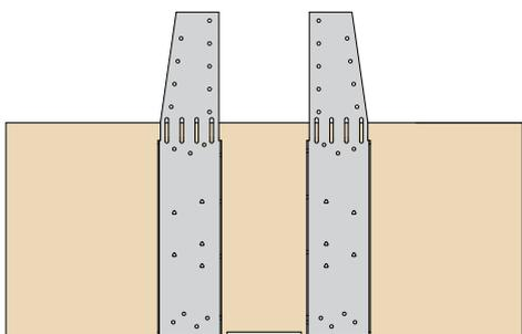
Position hanger flush with underside of joist.
