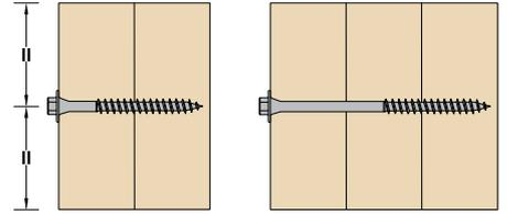
Figure 2 – Bottom Chords Depths of 122mm, 147mm, 172mm, 197mm or 222mm
