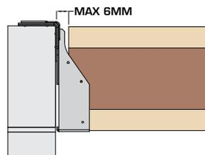
Do not install the hanger with a gap exceeding 6mm between the joist/truss and the hanger.
