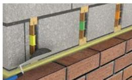
Add mortar to void created between block, joist and Hi-Vis Gripper and flush up.
