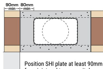
Position SHI plate at least 90mm from joist end to ensure it does not clash with masonry hanger or end seal (suitable for use with Hi-Vis Gripper).
