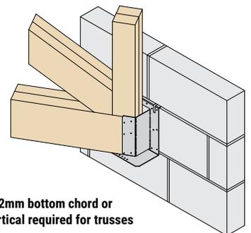
222mm bottom chord or vertical required for trusses
