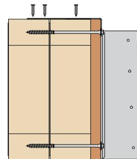
Nail top tabs into top chord of joist – Min 2No 3.4 x 35mm square twist nails into rear ply and 1No 3.4 x 35mm square twist nail into front ply per leg.
