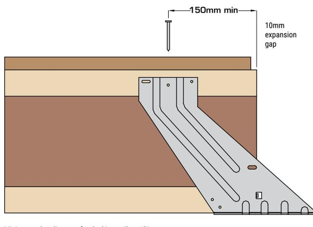
Minimum edge distance for decking nails = 150mm
