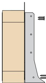
Face nail to top and bottom chords using 8No 3.4 x 35mm square twist nails in total.
