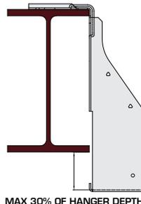
Where hanger extends past bottom of steel flange the drop must not exceed 30% of the hanger depth to prevent rotation.
