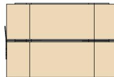
Position second ply of multiple joist on top of the OW-Clips and tap together with a hammer to ensure a tight fit.
