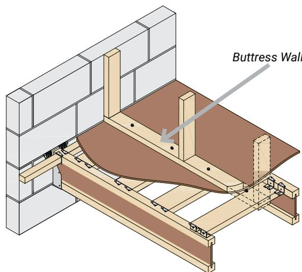
Noggins are evenly spaced between the joists (excluding perimeter noggin) and installed using UZ clips.
