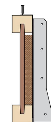
Wipe over top tabs to give a flush fit to the joist.
