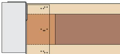
Web stiffeners required for I-Joists
