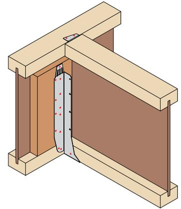
Offer incoming member into the UH hanger and fix to joist bottom flange/backer block and UZ-Clip to header member.
