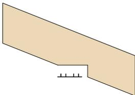
Tap bearing plate into position on underside of truss bearing area
