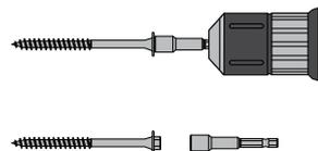
Install using an impact driver.
