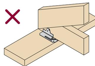
Do not install truss clips horizontally onto the wall plate.
