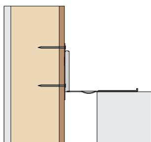
Once the channel is in position fix the top round hole into the wall panel, position the tie and build the next course of block work.
