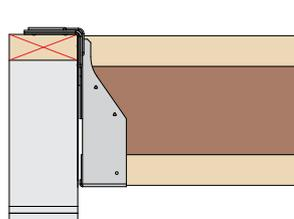
Do not install the hanger onto a timber wall plate.
