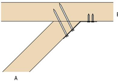
Joist A – 3.75 x 75mm round wire nails
