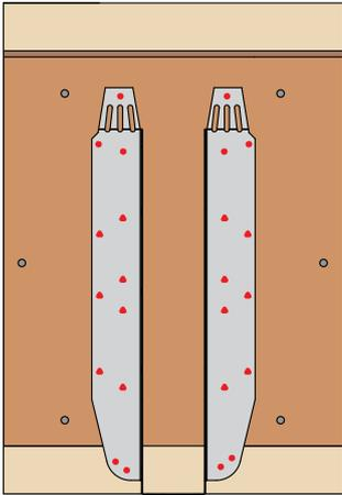
Position hanger against face of I-Joist with locating tab tight to underside of joist.
