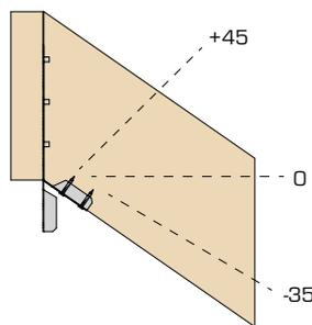
Offer incoming member and fix using 2No 3.4 x 35mm square twist nails to the underside of the incoming member.
