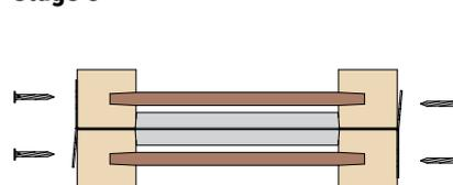
Fix I-Clips to top and bottom flanges of multiple I-Joist using 6No 3.4 x 35mm square twist nails ensuring that I-Joists are fitted tightly together.
