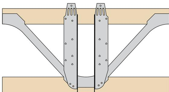
Position hanger against face of open web joist with locating tab tight to underside of joist.
