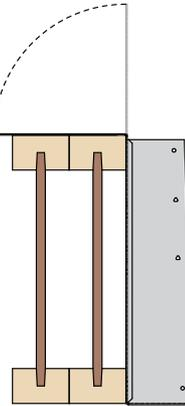
Wipe over top tabs to give a flush fit to the joist.
