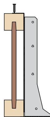
Nail top tabs into top flange of joist – 1No 3.4 x 35mm square twist nail per tab.
