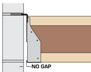
Do not install the hanger with a gap between the hanger and the face of the block work.
