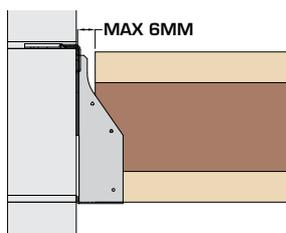
Do not install the hanger with a gap exceeding 6mm between the joist/truss and the hanger.
