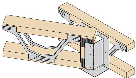
Please ensure that 1No inner nail hole (indicated in red) and 1No outer nail hole (indicated in red) are filled on the underside with 3.4 x 35mm square twist nails.
