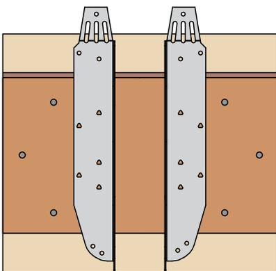
Position hanger against face of I-Joist with locating tab tight to underside of joist.
