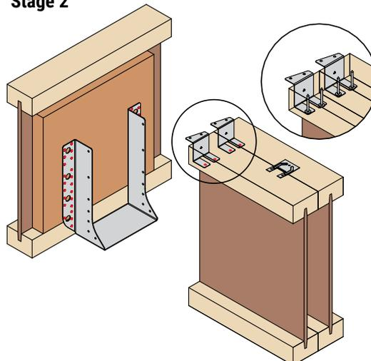
Fix UZ-Clips to top flange of supported member using:
