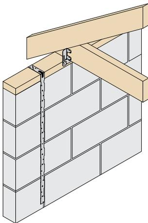
Fix VRS or LDGS to the wall plate with 2No 3.4 x 35mm square twist nails. Fixings into masonry to be specified by building designer.
