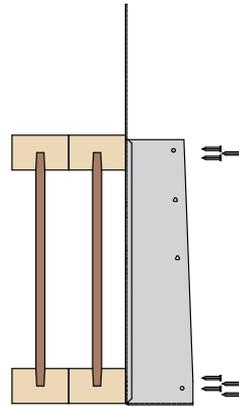
Face nail to top and bottom flanges using 14No 3.4 x 35mm square twist nails in total.
