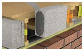
Lay mortar bed between joists, add mortar to perp end of block. Install block between joists tight to face of Hi-Vis Gripper.
