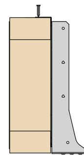
Nail top tabs into top chord of joist – 1No 3.4 x 35mm square twist nail per tab.
