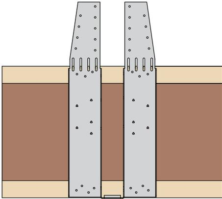
Position hanger flush with underside of joist.
