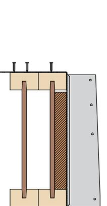
Nail top tabs into top flange of joist – Min 2No 3.4 x 35mm square twist nails into rear ply and 1No 3.4 x 35mm square twist nail into front ply per leg.
