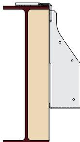
Where hanger does not extend past or rest on the bottom of the steel flange a timber packer is required to prevent rotation.
