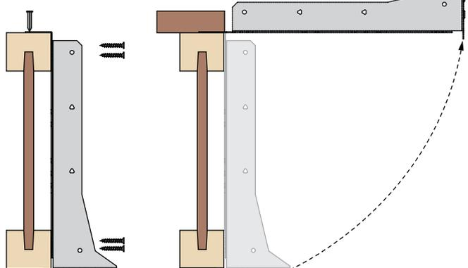
Face fix to top and bottom flanges using 8No 3.5 x 30mm multi purpose wood screws or 3.4 x 35mm square twist nails.
