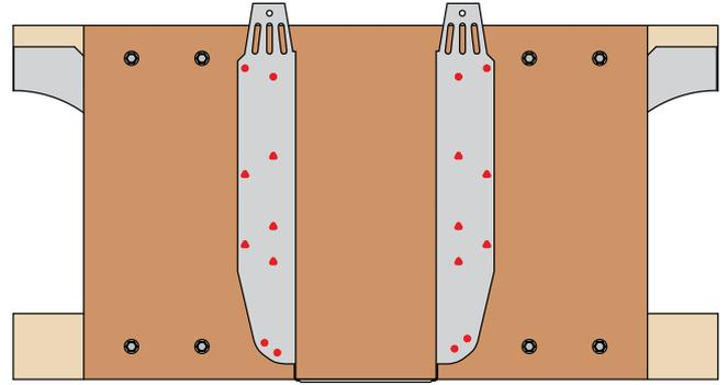
Position hanger flush with underside of joist.
