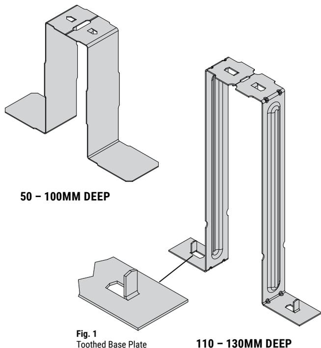
The IR-Clip allows for the use of high performance rigid insulation within a timber frame panel, whilst maintaining a service gap.
