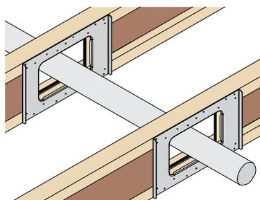
Plate required each side of aperture.
