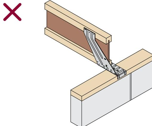
Do not install the RA range onto a timber wall plate.
