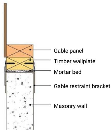
10mm maximum mortar bed on wall prior to wallplate being fixed.
