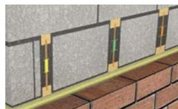
Ends of joist can be inspected to ensure correct installation before external brickwork built up.
