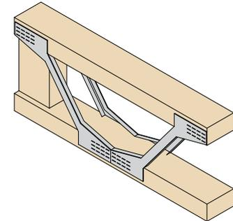
Do not use HUH for enhanced uplift when using trimmable ends
