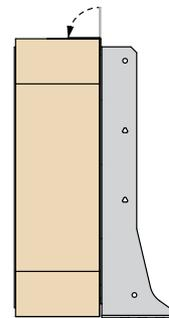
Wipe over top tabs to give a flush fit to the joist.
