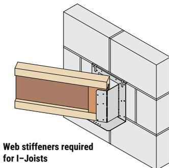
Web stiffeners required for I-Joists
