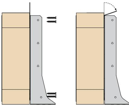
Face fix to top and bottom chords using 8No screws or nails.
