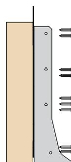
Fill all round and triangular nail holes to header with 3.4 x 35mm square twist nails.
