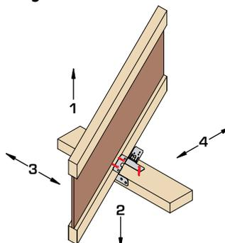
On the opposite side the ACE should be wiped up and nailed into the bottom flange with 2No 3.4 x 35mm square twist nails.
