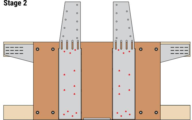
Position hanger flush with underside of joist.
