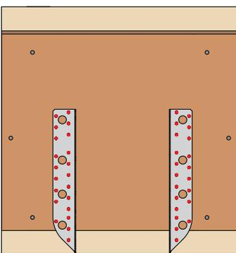
Position hanger against face of I-Joist with locating tab tight to underside of joist.
