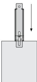
Position channel by lightly tapping with a hammer until channel is in correct position.
