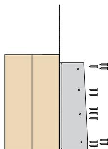
Fill all round and triangular nail holes to header joist with 3.4 x 35mm square twist nails.
