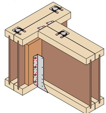
Offer incoming member into the MHE hanger and fix to joist bottom flange/backer block and UZ-Clip to header member.
