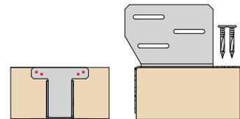
Nail to the top of the wall plate with 4No 3.4x35mm square twist nails
