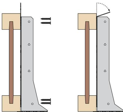
Face fix to top and bottom flanges using 8No 3.5 x 30mm multi purpose wood screws or 3.4 x 35mm square twist nails.
