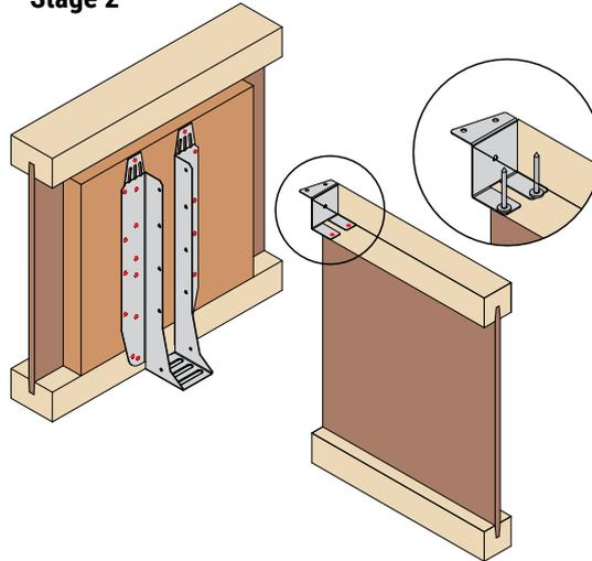
Fix UZ-Clip to top flange of supported member using:
