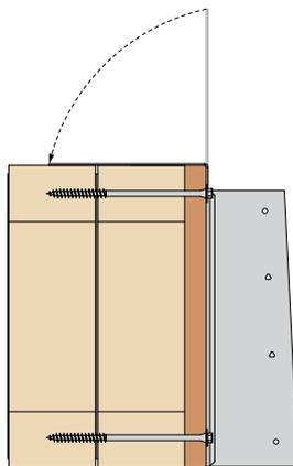
Wipe over top tabs to give a flush fit to the joist.
