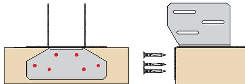
Position the slide shoe on the wall plate and nail to either face with 6No 3.4x35mm square twist nails
