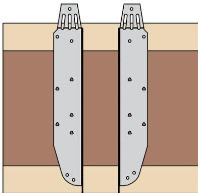
Position hanger against face of I-Joist with locating tab tight to underside of joist.
