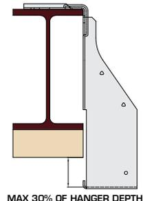
Where hanger extends past bottom of steel flange and drops >30% of the hanger depth a timber packer fixed as per building designers details can be used to reduce drop depth to <30%.
