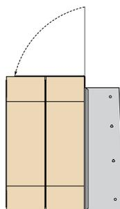
Wipe over top tabs to give a flush fit to the joist.
