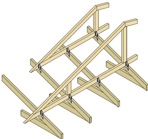
TA is to be installed on every occurring truss per valley truss.
