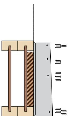
Fill all round and triangular nail holes to header and backer face with 3.4 x 35mm square twist nails.
