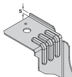
Do not flatten the 5mm upstands on the hanger top flanges. These are critical to the performance.
