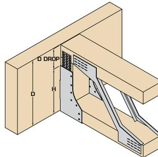
Applies to MHE/MHI/MHIC – Hanger height (H) must be minimum 60% of joist depth (D).
