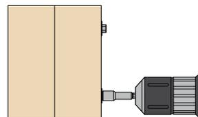
Bring the underside of the washer head flush with the timber surface.
