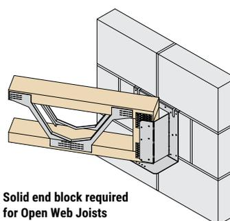
Solid end block required for Open Web Joists
