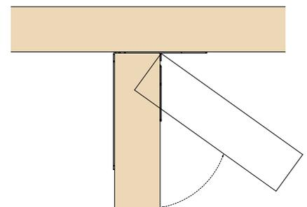
Rotate hanger to angle required. Correct hand must be used.
