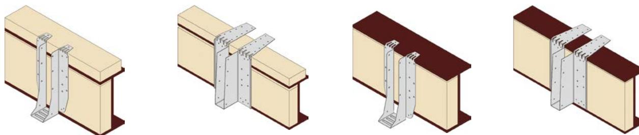
Hanger fixed to timber packer secured to top flange and web of steel beam using 3.4 x 35mm square twist nails. Timber packer fixed to web of beam (as per Building Designers instructions) to prevent hanger rotation. Timber packers must be a minimum of 35 x 72mm C16 grade timber.
