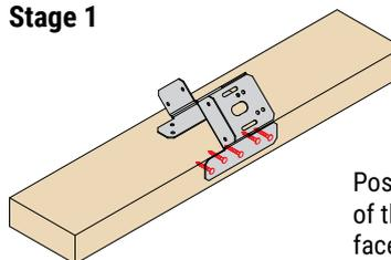
Position the ACE to the outside of the wall plate and nail to the face with 5No 3.4 x 35mm square twist nails.
