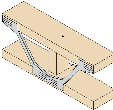
Applying a high load to the top flange of an open web joist can lead to failure of the joist itself (i.e metal webs buckling)
