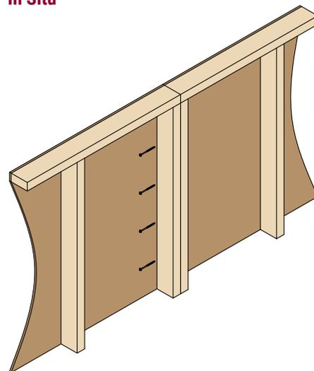
PSTS to be fixed at panel joints to engineer's specification.
