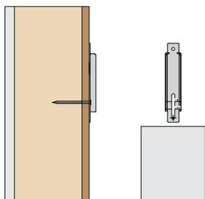
Nail channel into wall panel by nailing 1No fixing at the bottom of the slot. Allow adequate space above the masonry to hammer fix.
