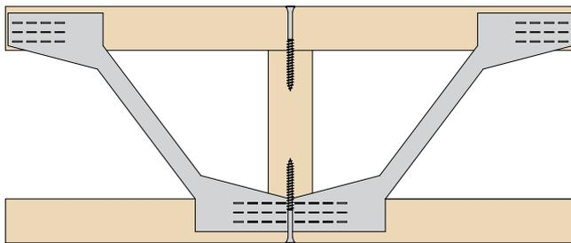
Vertical blocking piece to be built into Open Web Joist, centred on incoming hanger position.
