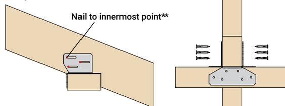
Nail through side flanges into the rafter with 6No 3.4x35mm square twist nails
