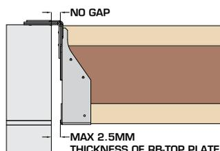
Do not install the hanger with a gap between the hanger and the face of the block work.
