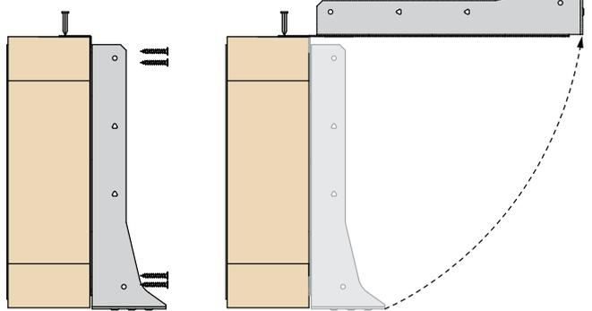
Face fix to top and bottom chords using 8No screws or nails.
